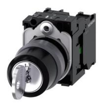
RONIS key-operated switch, 22 mm, round, plastic with metal front ring, lock number SB30, with 2 keys, 3 switch positions I-O-II, latching, actuating angle 2x45°, 10:30h/12h/13:30h, Key removal I+O+II, with holder, 1 NO, 1 NO, screw terminal, Z=20-unit packaging
