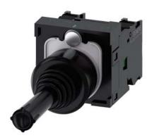
Coordinate switch, 22 mm, round, plastic, black, 2 switch positions, vertical latching, without mechanical interlocking, in O position, with holder, 1 NO, 1 NO, screw terminal, with laser labeling, inscription or symbol, Customer-specific selection with SIRIUS ACT configurator (CIN)
