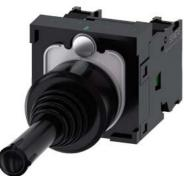
Coordinate switch, 22 mm, round, plastic, black, 2 switch positions, vertical, momentary contact type, without mechanical interlocking in O position, with holder, 1 NO, 1 NO, screw terminal, with laser labeling, upper case and lower case, always upper case at the beginning of the word
