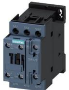
power contactor, AC-3e/AC-3, 38 A, 18.5 kW / 400 V, 3-pole, 24 V AC, 50 Hz, auxiliary contacts: 1 NO + 1 NC, screw terminal, size: S0
