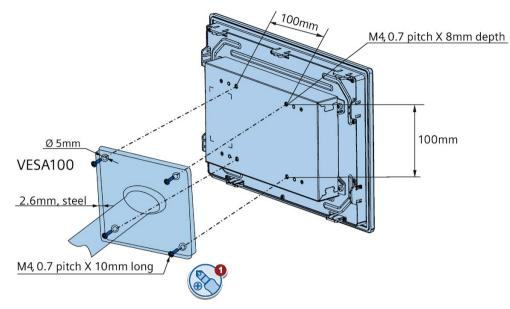
For the device SIMATIC IFP1200 Basic C, the VESA mounting is shown as follows:
