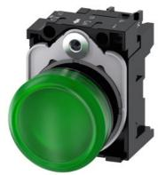
Indicator lights, 22 mm, round, plastic, green, lens, smooth, with holder, LED module, with integrated LED 230 V AC, screw terminal  $\,$
