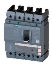
circuit breaker 3VA5 UL frame 250 breaking capacity class M 35kA @ 480 V 4-pole, line protection TM230, FTAM, In=125A overload protection Ir=125A fixed short-circuit protection Ii=5...10 x In N conductor protection 100% without connection
