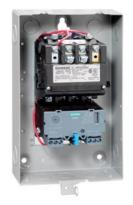
Non-reversing motor starter, Size 1, Three phase full voltage, Solid-state overload relay, OLR amp range 5.5-22A, Non-combination type, Enclosure type 1, Indoor general purpose use, Standard width enclosure
