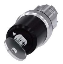
key-operated switch Siemens, 22 mm, round, metal, shiny, lock no. LSG1, with 2 keys, 2 switch positions O-I, latching, actuating angle 90°, 10:30h/13:30h, key removal O, with laser labeling, inscription or symbol customer-specific selection with SIRIUS ACT configurator (CIN)
