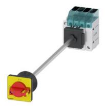
Load disconnector 3LD3, Iu 63 A Main switch 3-pole + N Rated operating capacity at AC-23 A at 400V 22.0 kW floor mounting Basic switch with door coupling Central hole mounting 22.5mm Toggle drive red / yellow 48x48 mm with auxiliary switch 1OE + 1S
