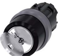
RONIS key-operated switch, 22 mm, round, plastic with metal front ring, lock number SB30, with 2 keys, 2 switch positions O-I, latching, actuating angle 90°, 10:30h/13:30h, key removal O+I, possible special locks: SB31, 421, 455, with laser labeling, lower case
