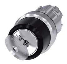
RONIS key-operated switch, 22 mm, round, metal, shiny, lock number SB30, with 2 keys, 2 switch positions O-I, latching, actuating angle  $90^\circ$ , 10:30h/13:30h, key removal O+I, possible special locks: SB31, 421, 455
