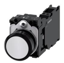
Pushbutton, 22 mm, round, plastic, white, pushbutton, flat, momentary contact type, with holder 1 NO+1 NC, spring-type terminal,
