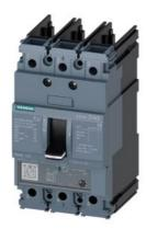
circuit breaker 3VA5 UL frame 125 breaking capacity class S 25kA @ 480V 3-pole, line protection TM230, FTAM, In=110A overload protection Ir=110A fixed short-circuit protection Ii=5...10 x In without connection
