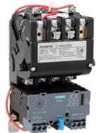
Non-reversing motor starter Size 1 Three phase full voltage Solid-state overload relay OLRelay amp range 10-40a 110-120/220-240VAC 60HZ coil Combination type No enclosure
