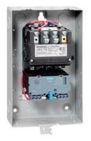
Non-reversing motor starter, Size 1, Three phase full voltage, Solid-state overload relay, OLR amp range 10-40A, Non-combination type, Enclosure type 1, Indoor general purpose use, Standard width enclosure
