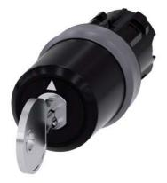
key-operated switch Siemens, 22 mm, round, plastic with metal front ring, lock number SSG10, with 2 keys, 3 switch positions I>O<II, momentary contact on the left, latching on the right, actuating angle 2x45°, 10:30h/12h/13:30h, key removal O, with laser labeling, upper case
