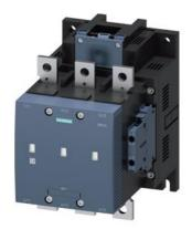
vacuum contactor AC-3e/AC-3 265 A, 132 kW / 400 V, 3-pole, Uc: 21-27.3 V AC(50-60 Hz) / DC PLC input 24 V DC drive: electronic auxiliary contacts 2 NO + 2 NC main circuit: busbar control and auxiliary circuit: screw terminal
