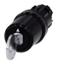
key-operated switch Siemens, 22 mm, round, plastic, lock number SSG10, with 2 keys, 3 switch positions I-O-II, latching, actuating angle 2x45°, 10:30h/12h/13:30h, key removal I+II
