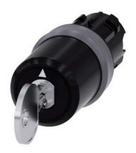
key-operated switch Siemens, 22 mm, round, plastic with metal front ring, lock number SSG10, with 2 keys, 3 switch positions I>O<II, momentary contact on the left, latching on the right, actuating angle  $2x45^\circ$ , 10:30h/12h/13:30h, key removal II, with laser labeling, inscription or symbol customer-specific selection with SIRIUS ACT configurator (CIN)
