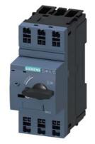
Circuit breaker size S00 for starter combination Rated current 8 A N-release 104 A Spring-type terminal Standard switching capacity
