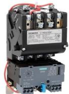
Non-reversing motor starter Size 1 Three phase full voltage Solid-state overload relay OLRelay amp range 0.75-3.4A 550/575-600 50/60HZ coil Combination type No enclosure
