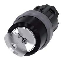
RONIS key-operated switch, 22 mm, round, plastic with metal front ring, lock number SB30, with 2 keys, 2 switch positions O-I, latching, actuating angle 90°, 10:30h/13:30h, key removal O, possible special locks: SB31, 421, 455, with laser labeling, lower case
