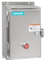
Non-reversing motor starter, Size 2 1/2, Three phase full voltage, Amb. compensate bimetal OLR, Contactor amp rating 60A, Non-combination type, Encl. type 4X 304 S. Steel, Water/dust tight noncorrosive
