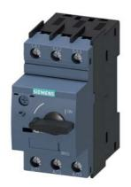
Circuit breaker size S00 for motor protection, CLASS 10 A-release 1.1...1.6 A N-release 21 A screw terminal Standard switching capacity
