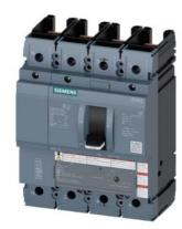
circuit breaker 3VA5 UL frame 250 breaking capacity class M 35kA @ 480 V 4-pole, line protection TM210, FTFM, In=125A overload protection Ir=125A fixed short-circuit protection Ii=10 x In N conductor protection 100% without connection
