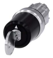
key-operated switch Siemens, 22 mm, round, metal, shiny, lock number SSG10, with 2 keys, 3 switch positions >0<II, momentary contact on the left, latching on the right, actuating angle  $2x45^{\circ}$ , 10:30h/12h/13:30h, key removal O, with laser labeling, upper case
