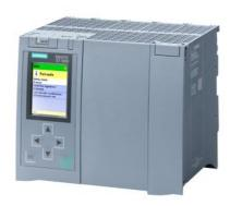
SIMATIC S7-1500TF, CPU 1518TF-4 PN/DP, central processing unit with 9 MB work memory for program and 60 MB for data, 1st interface: PROFINET IRT with 2-port switch, 2nd interface: PROFINET RT, 3rd interface: PROFINET basic services, 4th interface: PROFIBUS, 1 ns bit performance, SIMATIC memory card required
