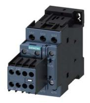
power contactor, AC-3e/AC-3, 25 A, 11 kW / 400 V, 3-pole, 125 V DC, auxiliary contacts: 2 NO + 2 NC, screw terminal, size: S0, removable auxiliary switch
