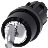
RONIS key-operated switch, 22 mm, round, plastic, lock number SB30, with 2 keys, 3 switch positions I>O<II, momentary contact on the left, latching on the right, actuating angle 2x45°, 10:30h/12h/13:30h, key removal O, possible special locks: SB31, 421, 455, with laser labeling, upper case and lower case, always upper case at the beginning of the word
