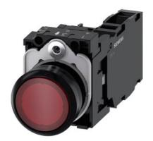
Illuminated pushbutton, 22 mm, round, plastic, red, pushbutton, flat, momentary contact type, with holder, 1 NO+1 NC, LED module with integrated LED 110 V AC, screw terminal, with laser labeling, upper case
