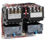
2-speed 3-phase motor starter Size 1 One winding consequent pole Constant or variable torque Solid-state overload relays Low SPD OLR range 3-12A High SPD OLR range 3-12A 110V 50HZ / 120V 60HZ coil Enclosure NEMA type (open) No enclosure
