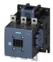
power contactor, AC-3e/AC-3 265 A, 132 kW / 400 V AC (50-60 Hz) / DC Uc: 110-127 V 3-pole, auxiliary contacts 2 NO + 2 NC drive: conventional main circuit: busbar control and auxiliary circuit: screw terminal
