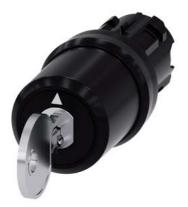
key-operated switch Siemens, 22 mm, round, plastic, lock number SSG10, with 2 keys, 3 switch positions I-O-II, latching, actuating angle 2x45°, 10:30h/12h/13:30h, key removal I+O+II, with laser labeling, upper case
