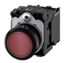
Illuminated pushbutton, 22 mm, round, plastic, red, pushbutton, flat, momentary contact type, with holder, 1NC, LED module with integrated LED 110 V AC, screw terminal, with laser labeling, symbol number according to, ISO 7000 or IEC 60417
