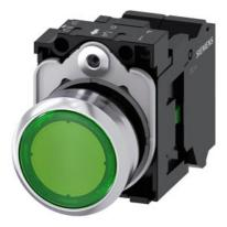
Illuminated pushbutton, 22 mm, round, metal, shiny, green, pushbutton, flat, momentary contact type, with holder, 1 NO, LED module with integrated LED 230 V AC, Spring-type terminal
