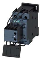
capacitor contactor, AC-6b 25 kVAr, / 400 V, 3-pole, 110 V AC, 50 Hz / 120 V, 60 Hz, auxiliary contacts: 1 NO + 2 NC, screw terminal, size: S0
