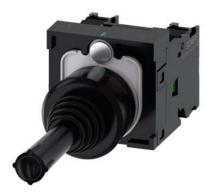
Coordinate switch, 22 mm, round, plastic, black, 2 switch positions, vertical latching, without mechanical interlocking, in O position, with holder, 1 NO, 1 NO, screw terminal, with laser labeling, upper case
