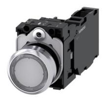
Illuminated pushbutton, 22 mm, round, metal, shiny, clear, pushbutton, flat, momentary contact type, with holder, 1 NO+1 NC, LED module with integrated LED 110 V AC, screw terminal, with laser labeling, inscription or symbol Customer-specific selection with SIRIUS ACT configurator (CIN)
