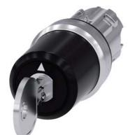
key-operated switch Siemens, 22 mm, round, metal, shiny, lock number SSG10, with 2 keys, 3 switch positions I>O<II, momentary contact on the left, latching on the right, actuating angle 2x45°, 10:30h/12h/13:30h, key removal O, with laser labeling, inscription or symbol customer-specific selection with SIRIUS ACT configurator (CIN)
