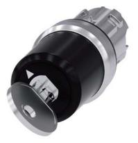
key-operated switch Siemens, 22 mm, round, metal, shiny, lock no. STGH10, with 2 keys, 2 switch positions O<I, momentary contact type, actuating angle 45°, 10:30h/12h, key removal O, with laser labeling, upper case and lower case, always upper case at beginning of line
