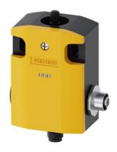
Basic switch without actuator head Metal enclosure, 56 mm wide ASIsafe integrated AS-i status: 1:F-IN1, 2: F-IN2 3:AS-i/FAULT Snap-action contacts 1 NC with M12 connector 4-pole Channel 1 to NC, Channel 2 to M12 socket on the right
