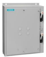
Duplex starter w/o alternator, Size 1, Three phase full voltage, Solid-state overload relay, OLR amp range 5.5-22A, 240V 50Hz / 277V 60Hz coil, Combination type, Two 25A circuit breakers, Enc NEMA type 4 painted steel, Water/dust tight for outdoors
