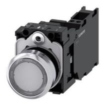
Illuminated pushbutton, 22 mm, round, metal, shiny, transparent, pushbutton, flat, momentary contact type, with holder, 1 NO+1 NC, LED module with integrated LED 230 V AC, spring-type terminal, Z=20-unit packaging
