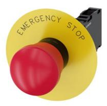
EMERGENCY STOP mushroom-type actuator, 22 mm, round, plastic, red, 40 mm, positive latching, according to EN ISO 13850, pull-to-unlatch mechanism, with yellow backing plate, inscription: EMERGENCY STOP, with holder, 1 NO+1 NC, screw terminal, Z=20-unit packaging
