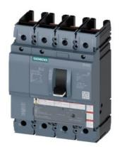
circuit breaker 3VA5 UL frame 250 breaking capacity class H 65kA @ 480V 4-pole, line protection TM210, FTFM, In=225A overload protection Ir=225A fixed short-circuit protection Ii=10 x In N conductor protection 100% without connection
