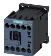
power contactor, AC-3e/AC-3, 9 A, 4 kW / 400 V, 3-pole, 24 V AC, 50/60 Hz, auxiliary contacts: 1 NC, screw terminal, size: S00
