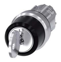
RONIS key-operated switch, 22 mm, round, metal, shiny, lock number SB30, with 2 keys, 3 switch positions I-O-II, latching, actuating angle 2x45°, 10:30h/12h/13:30h, Key removal II, possible special locks: SB31, 421, 455
