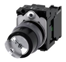
RONIS key-operated switch, 22 mm, round, plastic with metal front ring, lock number SB30, with 2 keys, 2 switch positions O-I, latching, actuating angle  $90^\circ$ , 10:30h/13:30h, key removal O+I, with holder, 1 NO, screw terminal, possible special locks: SB31, 421, 455, with laser labeling, inscription or symbol Customer-specific selection with SIRIUS ACT configurator (CIN)
