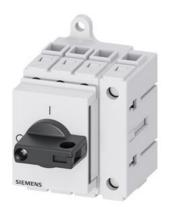
Load disconnector 3LD3, Iu 32 A Main switch 3-pole + N Rated operating capacity for AC-23 A at 400V 11.5kW Installation in distribution boards, Basic switch with selector knob black
